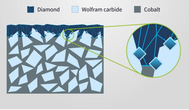
When coating with diamond, the proportion of cobalt in the carbide is of particular importance. It must neither be too large nor too small. CemeCon is happy to advise tool manufacturers on the selection of a suitable carbide on request.
