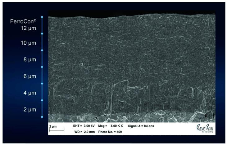
HiPIMS makes it possible: the dense layer structure is a quantum leap in coating for cutting tools
