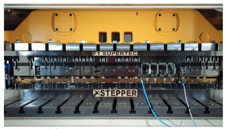
Modular progressive dies from Stepper can incorporate over 1,000 PVD-coated moving active parts, such as cutting punches, cutting, bending and embossing inserts. Excessive wear on any one of these active parts affects product quality. With HiPIMS technology, Stepper can significantly extend required maintenance intervals (typically to well over 10 million punch strokes without maintenance intervention).
