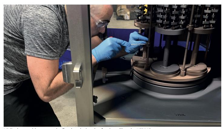
Mi-Tech was able to coat the first batch shortly after installing the HiPIMS system
