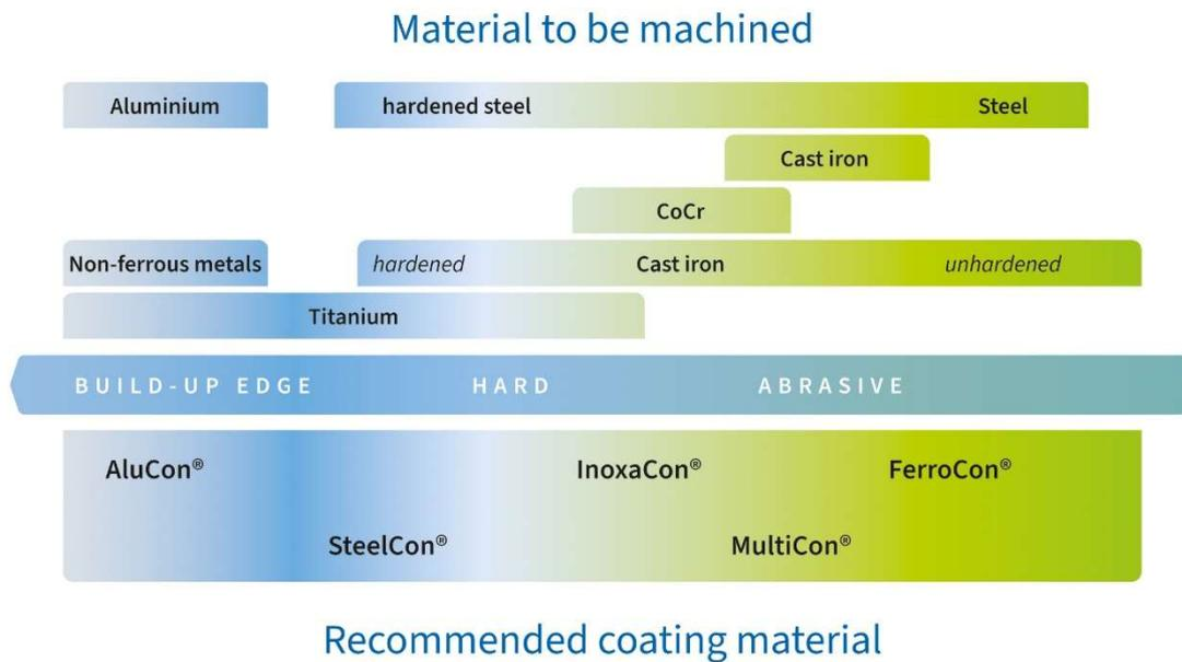
Hardened steel, stainless steel, cast iron or even titanium and aluminum - CemeCon always offers the right solution. With MultiCon®, CemeCon closes the gap between the HiPIMS coating materials FerroCon® and InoxaCon® for steel processing.
