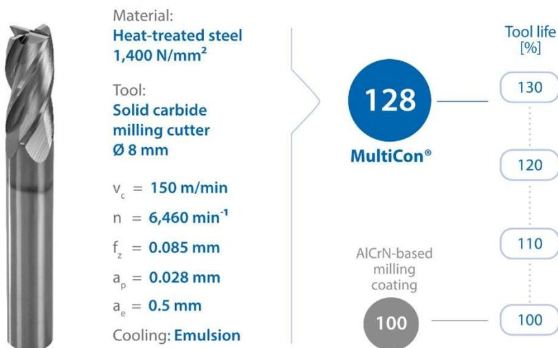
Practical examples show how MultiCon® increases productivity. When milling heat-treated steel (1,400 N/mm<sup>2</sup>), the tool life was increased by almost 30 percent compared to an AlCrN coating deposited using arc technology.
