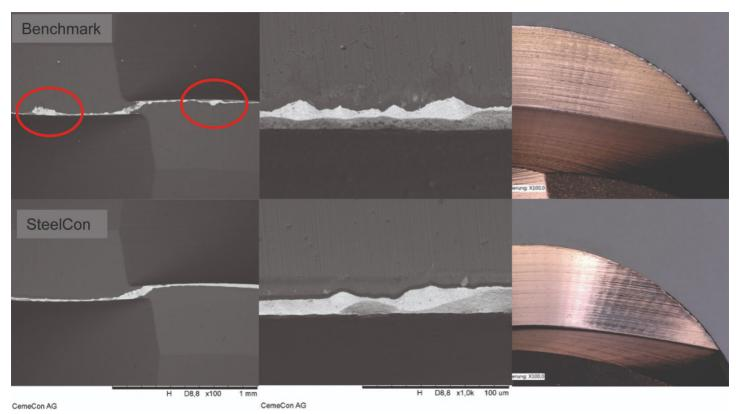
When milling hardened, alloyed stainless steel (1.2379) with a hardness of 62 HRC, the SteelCon®-coated tools exhibit significantly less wear than the Benchmark
