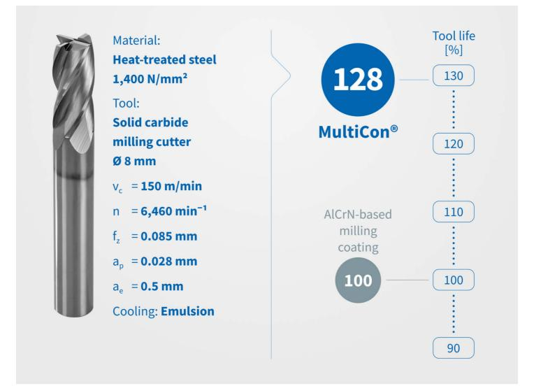
Practical examples show how MultiCon<sup>®</sup> increases productivity. When milling heat-treated steel (1,400 N/mm<sup>2</sup>), the tool life was increased by almost 30 percent compared to an AlCrN coating deposited using arc technology.
