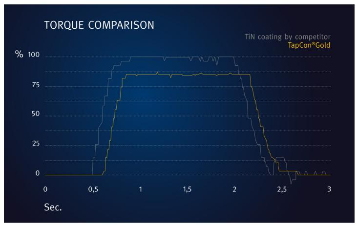
A stable low torque is enormously important for precise and efficient thread production. The newly developed HiPIMS coating material TapCon<sup>®</sup>Gold has been tailored specifically to these requirements and is the ideal coating base for HSS taps and thread formers.
