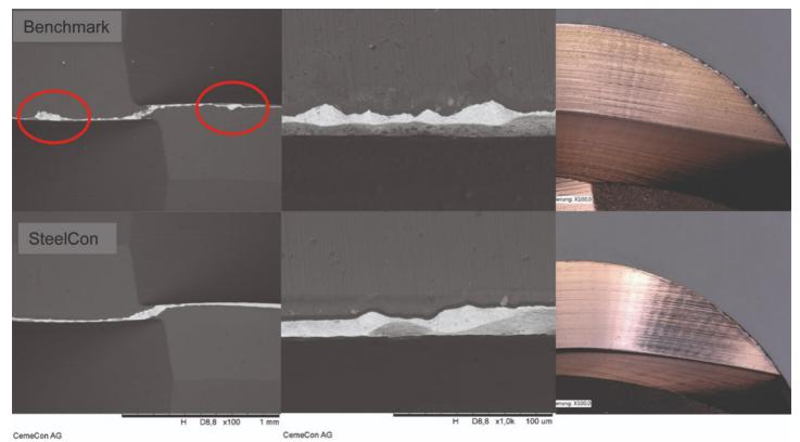
When milling hardened, alloyed stainless steel (1.2379) with a hardness of 62 HRC, the SteelCon<sup>®</sup>-coated tools exhibit significantly less wear than the Benchmark
