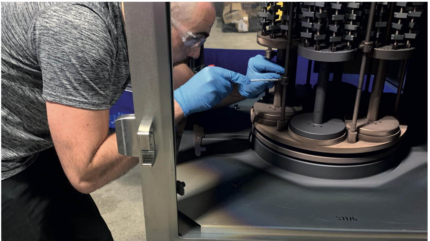
Mi-Tech was able to coat the first batch shortly after installing the HiPIMS system
